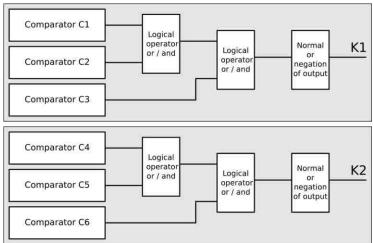
Picture 9. Comparators and logic functions
