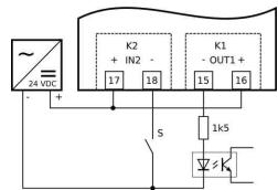
Picture 8: Connection of ENA33LCD input and output
