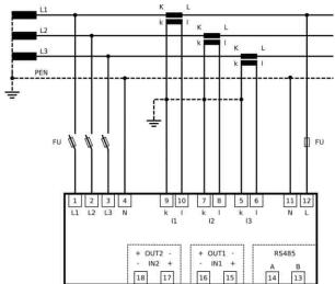
Picture 4. Three-phase measurement at TN-C network
