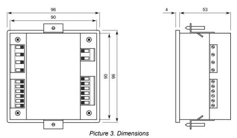
In order to assure well ventilation, instrument has to be installed vertically. There has to be empty space at least 50 mm at the top and bottom and 20 mm at the sides.
