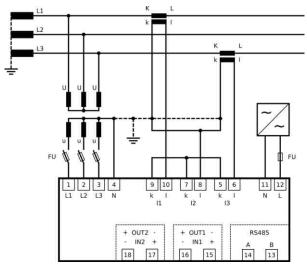
Picture 5. Connection at medium voltage network
