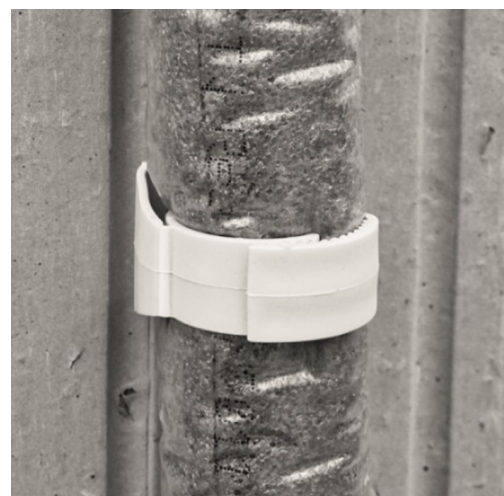
An innovative product for sub-plaster mounting - the Buried Clamp Automatic USA. A quick push is enough to affix the clamp to the pipe.
