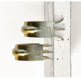
The C-Fix clip enables conduit to be mounted to plasterboard walls quickly and easily. The unique design ensures a strong grip and does not damage the outside of the wall. The flexible installation pipe is inserted into the CF, the CF is hit with a hammer - done!
