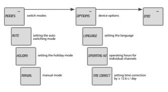
entrance into PRO programming menu browsing in menu 9/setting of values auick shifting during setting of values entrance into required (OK) menu confirmation one level up (ESC) a step back back to the starting menu
