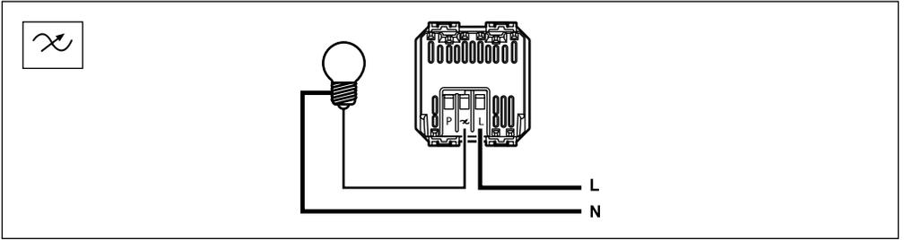
Diagram illustrating the remote control setup. The distance between the remote control and the light bulb is limited to 50 m max. The diagram shows a light bulb connected to a power source (L and N) through a switch mechanism. Below the diagram, there is a list of compatible models:
