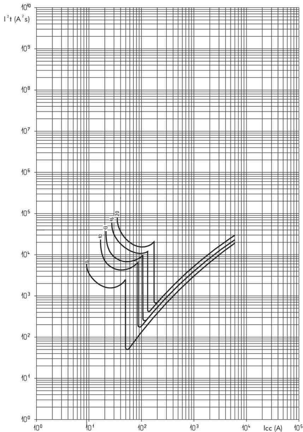
$I_{cc}$  = Prospective short-circuit symmetrical current (rms value in A) $I^2t$  = Limited thermal stress (in  $A^2 s$ )<sup>2</sup>
