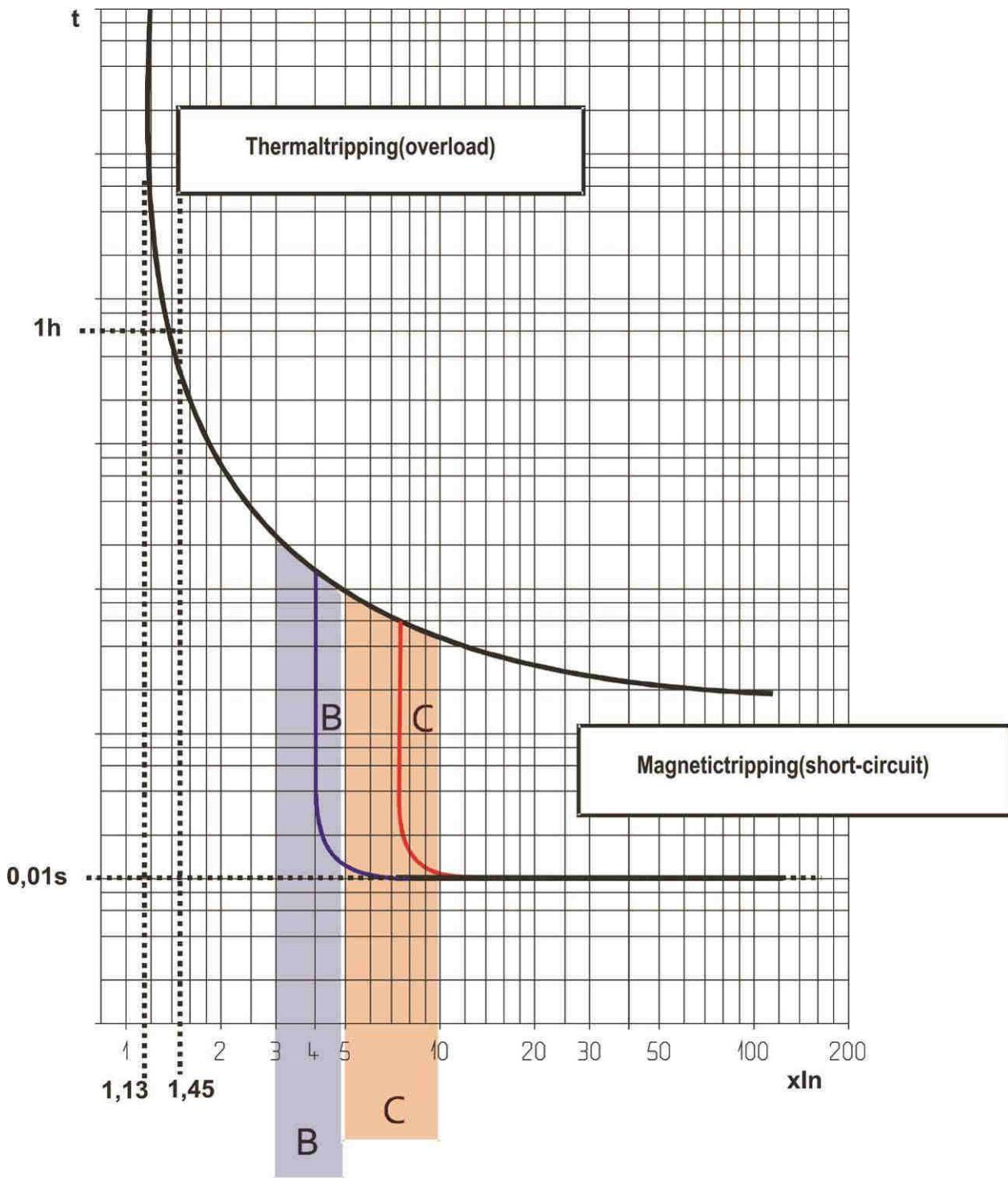
Thermal tripping at ambient temperature = 30°C
