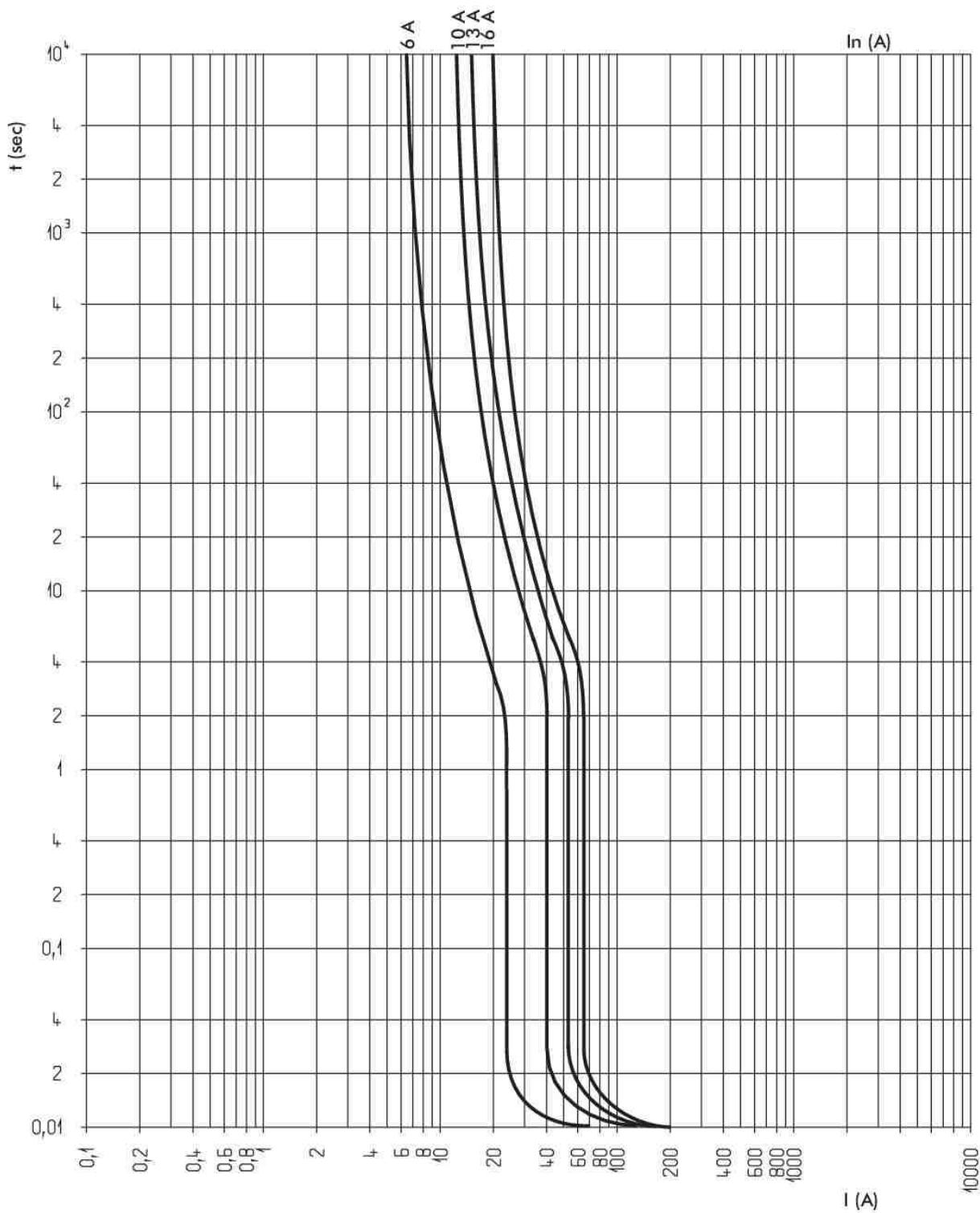
**Phase + Neutral, neutral on right side****7. CURVES (continued)****Average thermal-magnetic tripping curves range typical of C curve DX<sup>3</sup> STOP ARC:**
