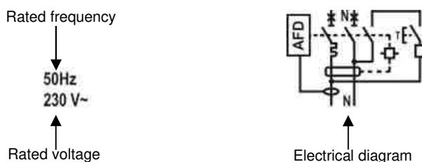
. The terminals upstream and downstream of the neutral pole are marked with an "N" moulded close to the screw heads.
