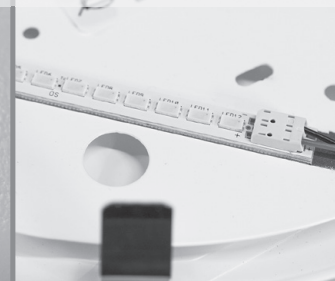
LED MODUL A CHLADIČ / LED MODULE, COOLING PLATE
