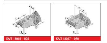
The chain bracket is a fully plastic part. The bracket is precisely adjusted to the respective chain width and only needs to be snapped in at the chain link. Please order one male and one female end bracket for each chain. The brackets should be fastened with M5 screws. The cables or conduits may be fastened with cable ties on the integrated strain relief of the chain bracket.
