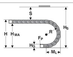
The moving end chain connection is to be screw fixed at height  $\rm H_{\rm \tiny MA}$  for the respective radius. For the installed dimension the "Installed height  $\rm H_{\rm s}$  " value has
