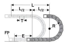
The fixed point of the cable drag chain should be connected in the middle of the travel distance.
