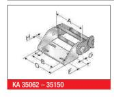
The metal connection (U-section) is precisely adjusted to the respective chain width. It only needs to be snapped in the chain link. Please order one male and one female end bracket for each chain. The brackets should be fastened with M6 screws.
