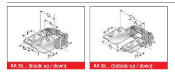
The chain bracket can be supplied either in galvanised sheet steel or stainless steel. To secure one cable drag chain, you will need two angle brackets (left and right) with a drilled hole and two angle brackets (left and right) with a bolt. The order numbers given below each comprise a left and right angle bracket.
