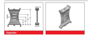
We recommend that separators be used if multiple round cables or conduits with differing diameters are to be installed.
