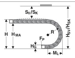
The moving end chain connection is to be screw fixed at height  ${\rm H}_{\rm {\tiny MA}}$  for the respective radius.
