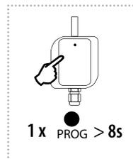
By pressing the programming button on the actuator for 8 seconds, deletion occurs of the actuator's entire memory. LED flashes 4x in each 1s interval.
