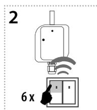
Assignment of the delayed on function is performed by six presses of the selected button on the RF transmitter (must be a lapse of 1s between individual presses).
