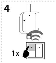
After the desired time has elapsed (range of 2s...60min), the timing mode ends by pressing the button on the RF transmitter, to which the delayed return function is assigned. This stores the set time interval into the actuator memory.
