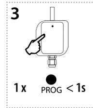
Press of programming button on receiver RFUS-61 shorter than 1 second will finish programming mode. The LED lights up according to the pre-set memory function.
