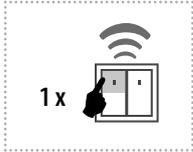
The output contact will be closed by pressing the button.
