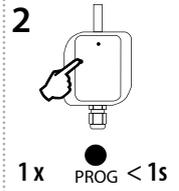
Pressing the programming button on the RFUS-61 receiver for less than 1 second will finish the programming mode, this will reverse the memory function. The LED lights up according to the current pre-set memory function. The set memory function is saved.
