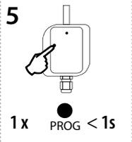
Press of programming button on receiver RFUS-61 shorter than 1 second will finish programming mode. The LED lights up according to the pre-set memory function.
