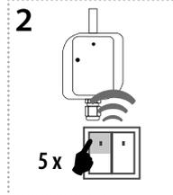
Assignment of the delayed off function is performed by five presses of the selected button on the RF transmitter (must be a lapse of 1s between individual presses).
