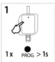
Press of programming button on receiver RFUS-61 for 1 second will activate receiver RFUS-61 into programming mode. LED is flashing in 1s interval.
