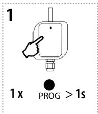
Press of programming button on receiver RFUS-61 for 1 second will activate receiver RFUS-61 into programming mode. LED is flashing in 1s interval.
