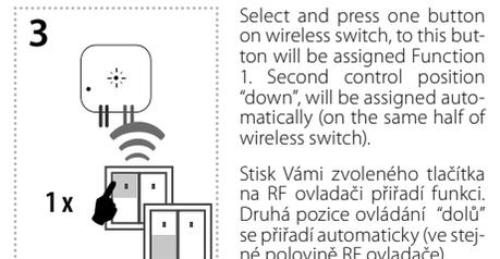
Select and press one button on wireless switch, to this button will be assigned Function 1. Second control position "down", will be assigned automatically (on the same half of wireless switch).
