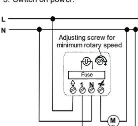
Via the terminals 1 and N the speed controller can be illuminated by a fuse unit with glow lamp (included or retrofit) Only in this case the connection of the neutral conductor (N) is necessary.
