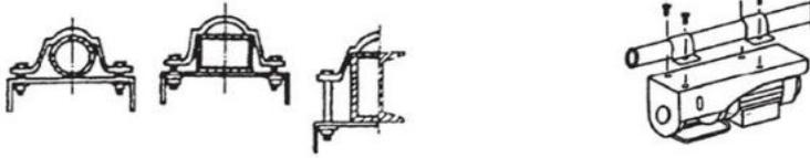
The carrier construction shall ensure a safety fixing for the carrier stirrups and provide the movement or the offset of the hoist. The construction shall also be able to withstand the static and dynamic actions occurring when manipulating the tool.
