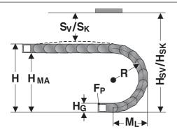
The moving end chain connection is to be screw fixed at height  $\mathbf{H}_{_{\mathrm{M}\Delta}}$  for the respective radius.
