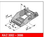
The type KA/Z 3001-3006 chain bracket is a plastic part with an extrusion-coated metal insert. The bracket is precisely adjusted to the respective chain width and only needs to be snapped in at the chain link. Please order one male and one female end bracket for each chain. The brackets should be fastened with M6 screws. The cables or tubes may be fastened with cable ties at the integrated strain relief of the chain bracket.
