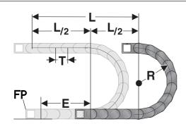
The fixed point of the cable drag chain should be connected in the middle of the travel distance.
