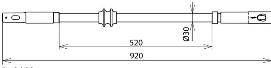
Insulating stick with plug-in coupling for operating head (hammer).
