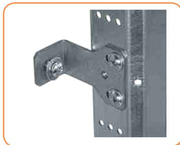
LG-V5 elements are used to fix the rails TH-S and mounting plates PM to vertical bracket WP-A. It is done with the help of two sheet metal screws (AST 4.8x9.5). The LG-V element contains a metric nut M5.
