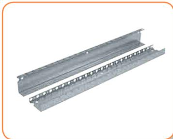
Vertical bracket economical version offers no possibility of the enclosure division and mounting depth TH-S rails adjustment as well as mounting plates PM. The same distance (48.5 mm) from rails TH-S to covers. Rails TH-S and plates PM are directly mounted to the bracket WP-U by means of sheet metal screws AST 4.8x9.5 without the use of fasteners LG-V. The brackets are attached to the enclosure with Allen screws M6x10 supplied along with the enclosure.
