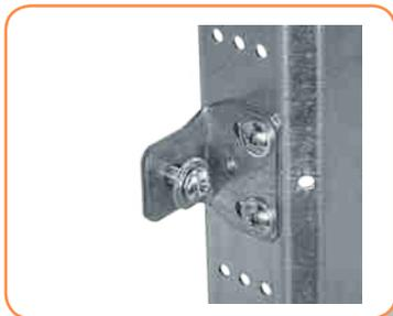
LG-V elements are used to fix the rails TH-S and mounting plates PM to vertical bracket WP-A. It is done with the help of two sheet metal screws (AST 4.8x9.5). The LG-V element contains a metric nut M5.
