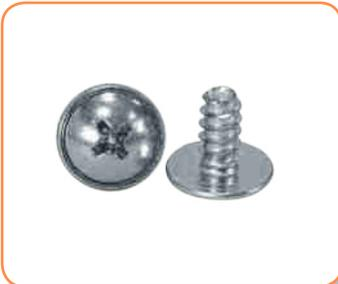
An important element of the system is a special sheet metal screw AST 4.8x9.5 with Philips head PH2. If is used to fix elements LG-V / LG-V5 to the s WP-A, WP-U, TH-S rails, mounting plates PM, cable glands covers in GT enclosures, back plates in XN.. enclosures
