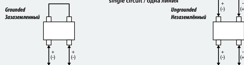
**1500Vdc : IEC 60947-3 - 1500Vdc : 98B - 600Vdc : CSA C22.2 Nr. 4 [3poles in series min. per circuit] / [3 pola v seriji]**
