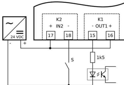
Picture 8: Connection of ENA33LCD input and output
