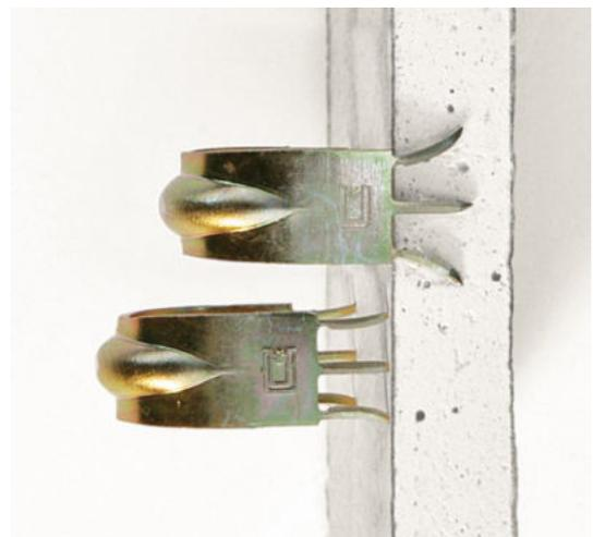
The C-Fix clip enables conduit to be mounted to plasterboard walls quickly and easily. The unique design ensures a strong grip and does not damage the outside of the wall. The flexible installation pipe is inserted into the CF, the CF is hit with a hammer - done!
