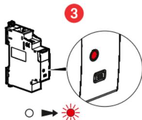
**3** Press and hold the Gateway module settings button, or in the center of the General Scenario Wireless Command until the LED turns green, then release the button.
