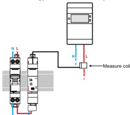
\*: Do not use on a three Lines electrical installation.
