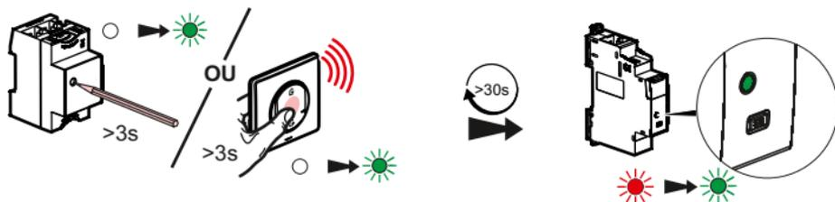
The configuration LEDs of " ... with Netatmo " devices must all light up in fixed green.
