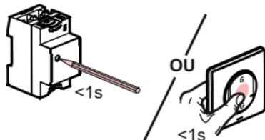
**Briefly press** the setting button on the Gateway module (or in the center of the General Scenario Wireless Command) to finalize the installation. All devices LED go OFF.
