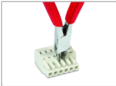
Coding a female connector – removing coding finger(s).
