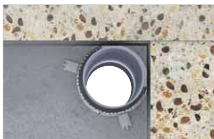
■ Suitable for corner penetrations ( \frac{2}{3} fire collar). Distance between wall and pipe \leq 10 mm.
