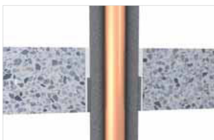
■ Non-combustible pipes with insulation into the floor.
