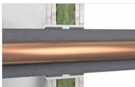
■ Non-combustible pipes with insulation into the wall.
