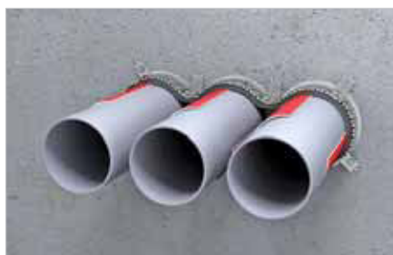
■ Multiple penetrations (max. 3 pipes through 1 Fire Collar). Distance between pipes \leq 15 mm.
