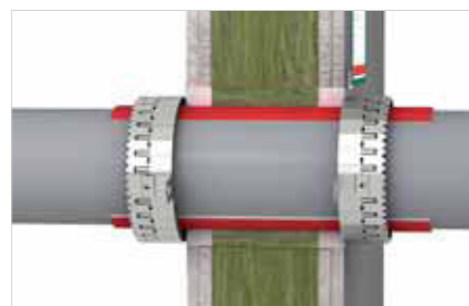
■ Penetration through metal stud wall sealed with loose mineral wool and Pacifyre® FPM Fire Protection Mortar.
