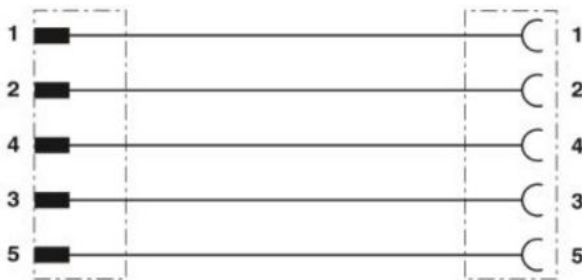
Pin assignment between M12-plug and M12-jack
