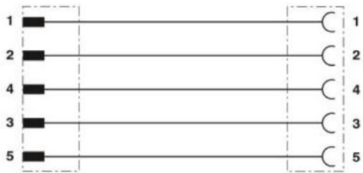
Pin assignment between M12-plug and M12-jack
