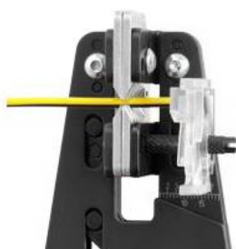
Put the cable on the length stop
