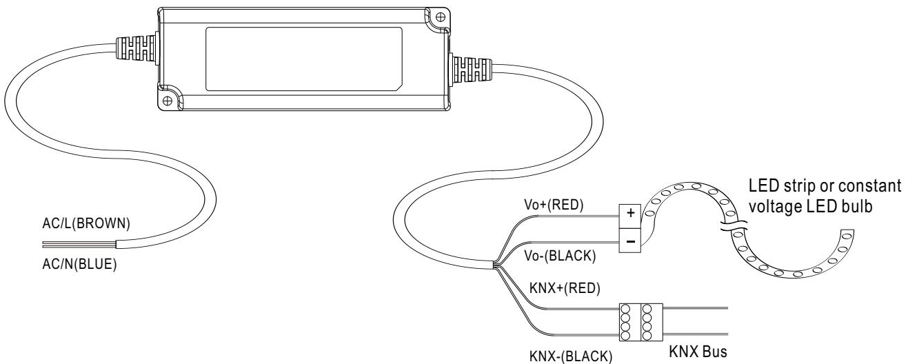
PWM KN series can be ETS addressing/programming WITHOUT connecting to AC mains
