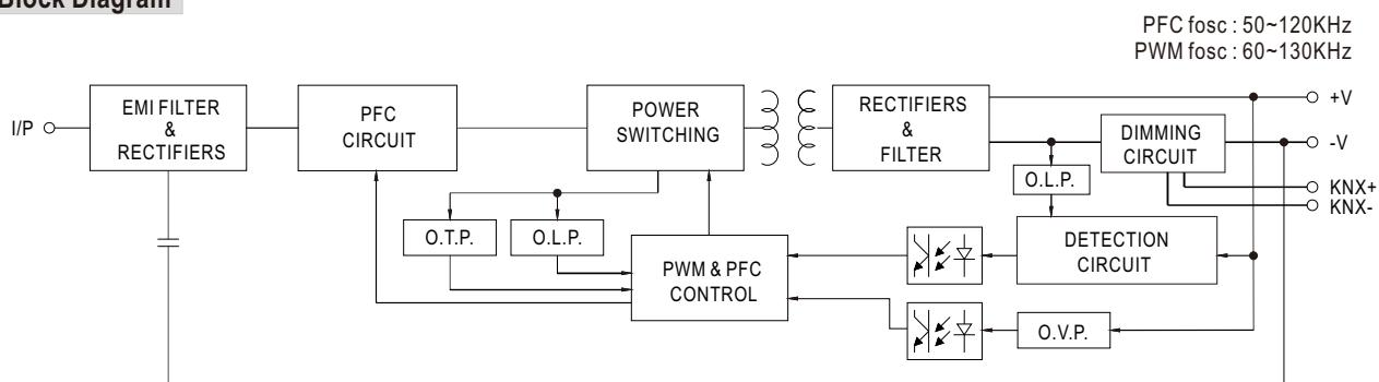
Note: PWM fosc here is not related to output PWM dimming
