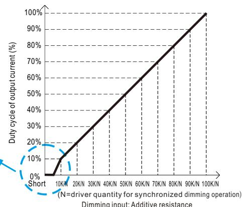
Note : 1. Min. duty cycle of output current is about 1%, and the dimming input is about 6KΩ or 0.6VDC, or 10V PWM signal with 6% duty cycle.
