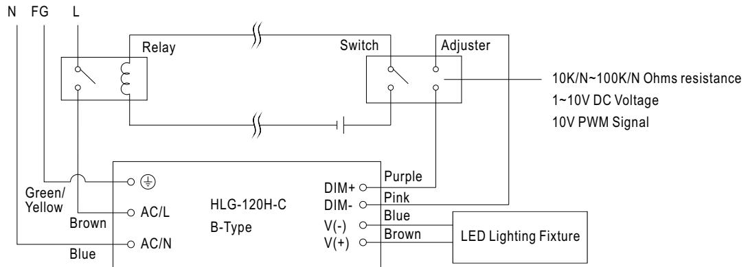
Using a switch and relay can turn ON/OFF the lighting fixture.
