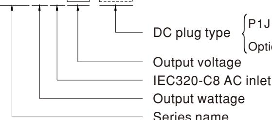
P1J: Plug for standard model, 2.1φ x 5.5φ x 11mm, c+, tuning fork type
