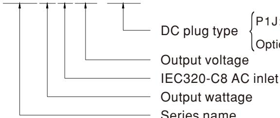
P1J: Plug for standard model, 2.1φ x 5.5φ x 11mm, c+, tuning fork type
