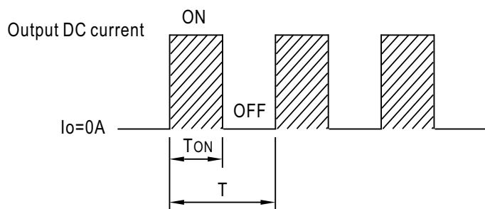
$$\text{Duty cycle(%)} = \frac{\text{TON}}{\text{T}} \times 100\%$$
