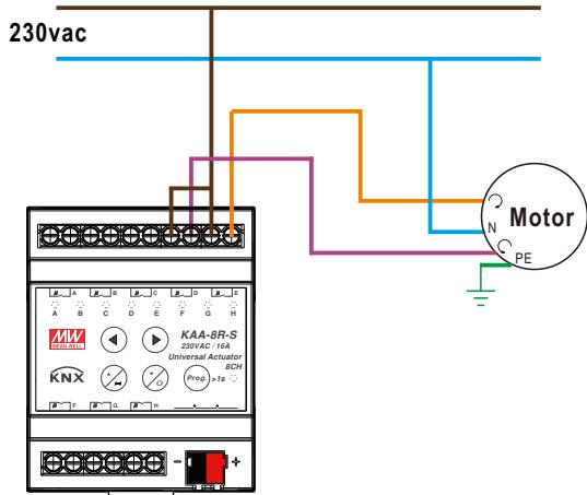
Note: Check installation manual of shutter motor for wiring.
