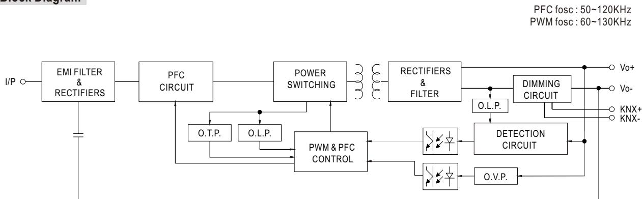
Note: PWM fosc here is not related to output PWM dimming
