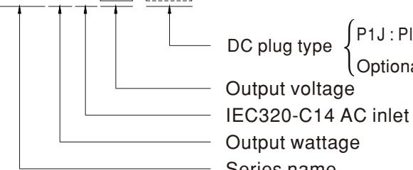
DC plug type { P1J : Plug for standard model, 2.1ψ x 5.5ψ x 11mm, c+, tuning fork type
