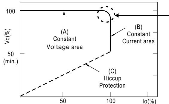
In the constant current region, the highest voltage at the output of the driver depends on the configuration of the end systems.
