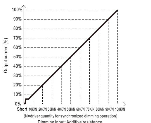
Note : 1. Min. dimming level is about 8% and the output current is not defined when 0% < Iout < 8%.
