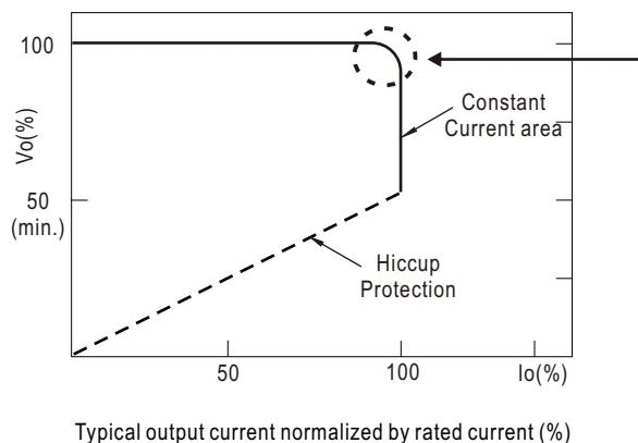
In the constant current region, the highest voltage at the output of the driver depends on the configuration of the end systems.
