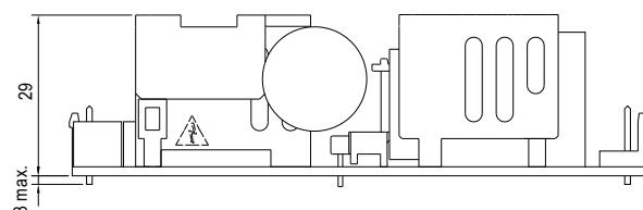
AC Input Connector (CN1) : JST B3P-VH or equivalent
