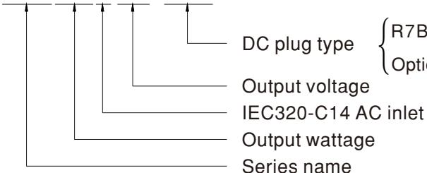
DC plug type      R7B: Plug for standard model, Power DIN 4Pin with lock type
