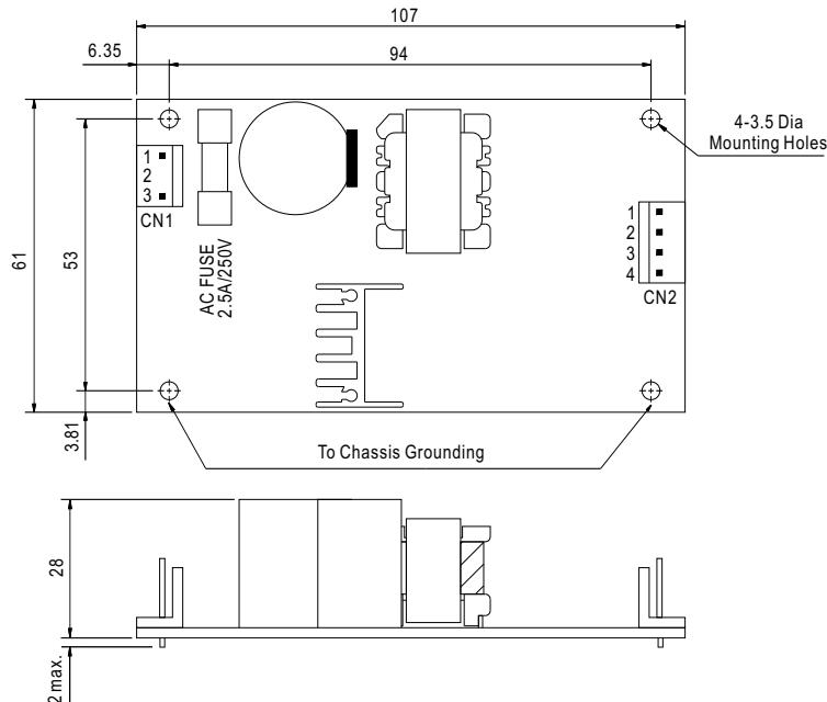
AC Input Connector (CN1) : Molex 41791-03 or equivalent
