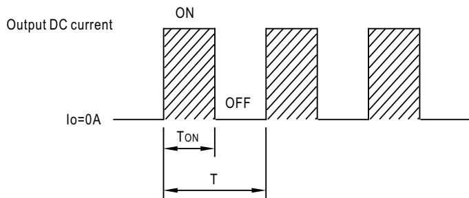
$$\text{Duty cycle}(\%) = \frac{T_{ON}}{T} \times 100\%$$
