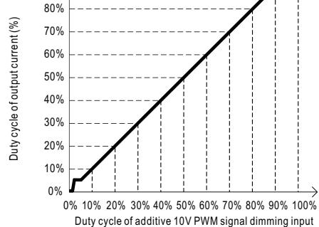
Note : 1. Min. duty cycle of output current is about 8% and the output current is not defined when  $0\% < I_{out} < 8\%$ .
