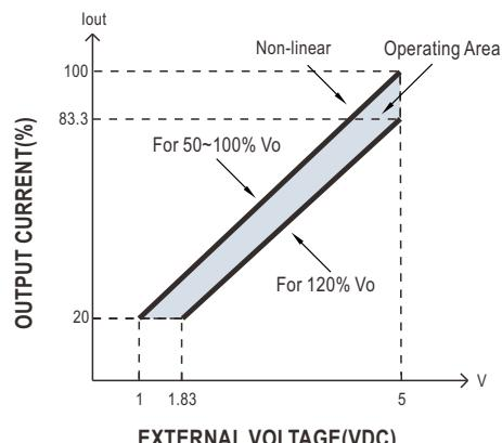
※ Caution: By factory default, the Output Current Programming is not activated, and VCCS(pin13) and PC-DIS(pin14) are shorted by connector. Whenever this function is not needed to activate, as assumed in other sections' diagrams, please keep VCCS(pin13) and PC-DIS(pin14) shorted ; otherwise, the power supply will have no output.
