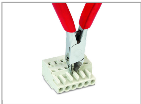
Coding a female connector – removing coding finger(s).
