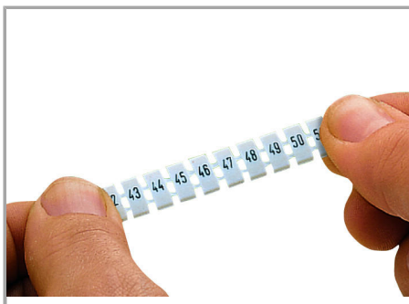
Stretching a WMB marker strip.
